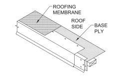
**STEP 3: Installing Approved Roofing Membrane** Install roofing membrane per manufacturer's instructions.
